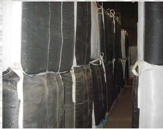
Ventilated FIBC's are stable when double stacked due to their square shape which maximizes warehouse utilization.
