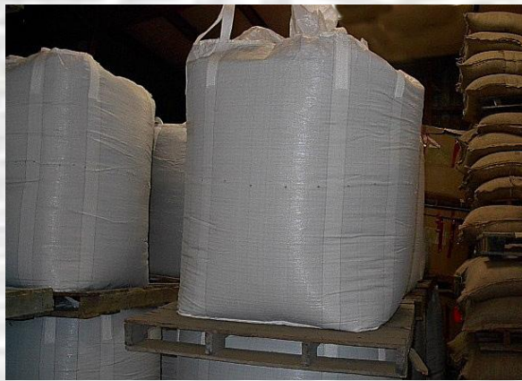
Unstable burlap bags and other packaging require extra handling while bulk bags provide greater stability, more capacity and ease of handling.
